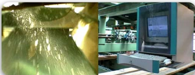
Saw dust damages PCs so industrial PCs with protective casings were required
