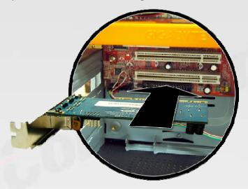
5. Replace the cover and reconnect all peripheral and power cables.
