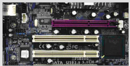
4. Insert the X300 PCI card and secure the end of the card to the chassis with a retaining screw. Note: If required, you can use the included low profile bracket.
